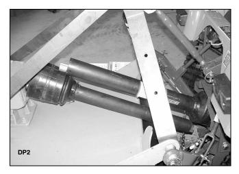
Figure 5. Drive Halves Placed Parallel
